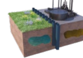
Cut-off walls in ecologically threatened areas
